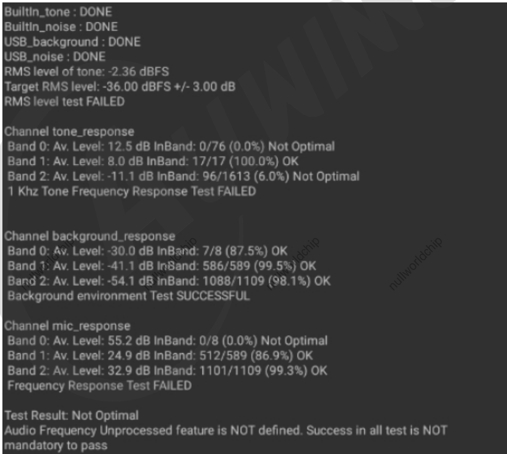
图 20: Audio Frequency Unprocessed Test 测试结果提示
