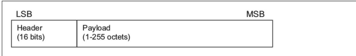
Figure 2.4: Advertising physical channel PDU
