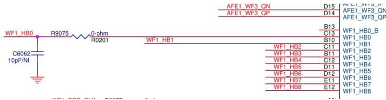
Fig 5-62 : WF0 HB0 is CLK keep other signal away
