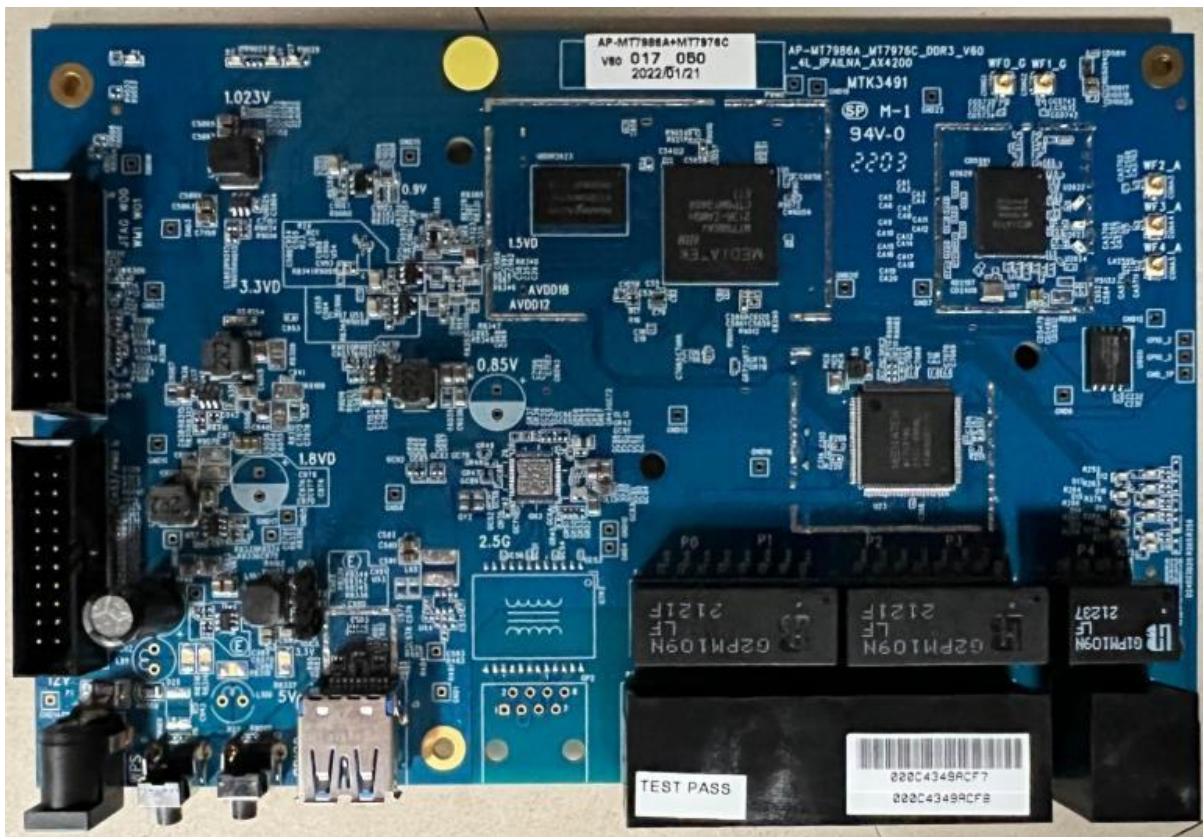
Fig 4-1: MT7986A+MT7986C RFB Top view
