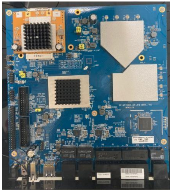
Fig 5-68 : Reserve shielding example
