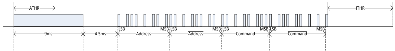
Figure 9-109 NEC Protocol
