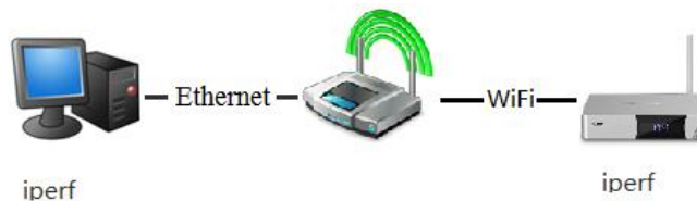
Figure 4-1 Networking for the throughput test
